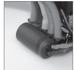
Mount the power-capacitor in a position where it is protected in the event of a crash. The best place is right next to the speed-control (see picture). Secure it with doublesided tape.
